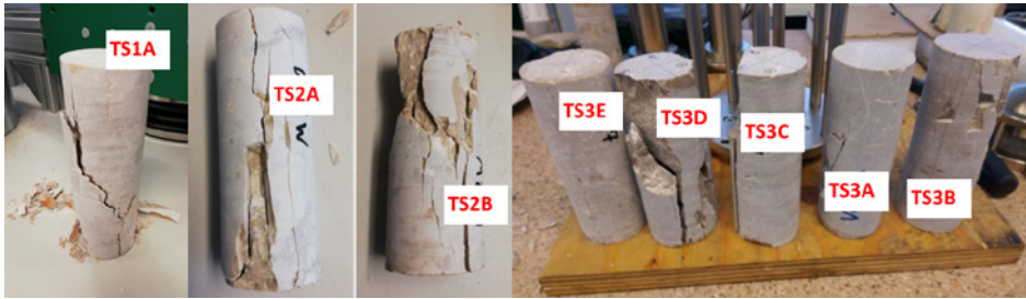
Figure 5. Tested specimens after failure in uniaxial compression
